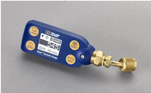
The OMNI Vacuum Gauge is rugged and built to last. Made with high impact, glass reinforced housing, it survives moisture and accidental drops or attachment to a high pressure line. The easy-to-clean vacuum sensor handles 450 psi positive pressure and reads several units of vacuum (microns, millibar, Torr and Pascal).
