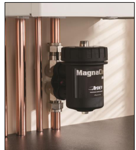
Figure 1: ADEY's MagnaClean Micro2 ™ is designed for small spaces. Housed inside the canister is a powerful permanent magnet that traps iron oxide, removing it from the system and preventing expensive damage.
